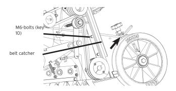
• Remove the two M6 bolts, nuts and washers and then lift the plate. Use a 10 mm ring spanner.
