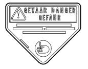
This sticker is affixed on the belt protection cover and warns about the danger of hand injuries. Keep your hands and feet away from underneath the machine as long as the blades are rotating. The engine must be turned off in case of faulty operation or before starting maintenance. Art nr : BQ 505 010 070
